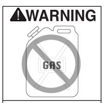
Never use use gasoline or other flammable liquids to clean this tool. Vapors in the tool may ignite, causing the tool to explode. Ignoring this warning may lead to serious personal injury or even death!
